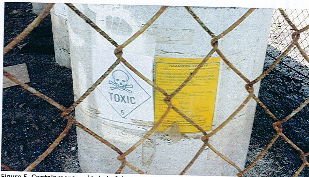
Figure 5. Containment and Label of the PCB Oil
